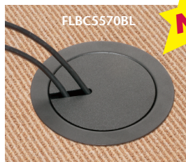
Cover options Install gasket and blank with #8-32 x 5/8" screws or install in-use cover (no screws required).
